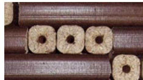
processes. The sawdust is compressed and the lignin contained in the wood can be softened, allowing it to act as a natural binder, producing a reformed log size product which should conform to European standard EN ISO 17225-3. Briquettes are dense which reduces the amount of storage space required and they're also clean to handle and easy to take home in 'ready to burn' retail packs.
