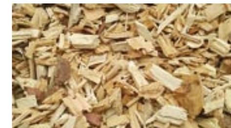
will help the appliance (especially domestic sized boilers) work at their optimum efficiency and reliability. Typical wood chip from a tree surgeon is too wet and variable in chip size for most appliances.
